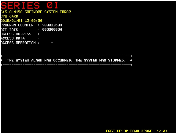
Example of system alarm screen
